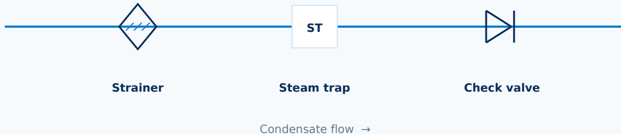
Figure 1 · Conceptual sequence of strainer, steam trap and check valve in a condensate line.
